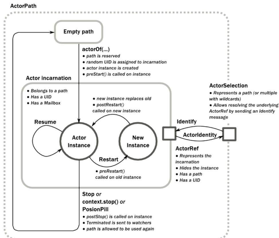
A path in an actor system represents a “place” which might be occupied by a living actor. Initially (apart from system initialized actors) a path is empty. When `actorOf()` is called it assigns an *incarnation* of the actor described by the passed `Props` to the given path. An actor incarnation is identified by the path *and a UID*. A restart only swaps the `Actor` instance defined by the `Props` but the incarnation and hence the UID remains the
