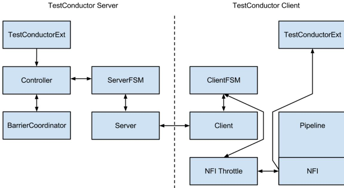
The test conductor server is responsible for coordinating barriers and sending commands to the test conductor clients that act upon them, e.g. throttling network traffic to/from another client. More information on the possible operations is available in the `akka.remote.testconductor.Conductor` API documentation.
