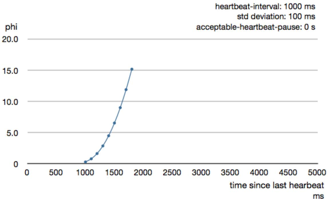
To be able to survive sudden abnormalities, such as garbage collection pauses and transient network failures the failure detector is configured with a margin, `akka.remote.watch-failure-detector.acceptable-heartbeat-pause`. You may want to adjust the *Remote Configuration* of this depending on you environment. This is how the curve looks like for `acceptable-heartbeat-pause` configured to 3 seconds.
