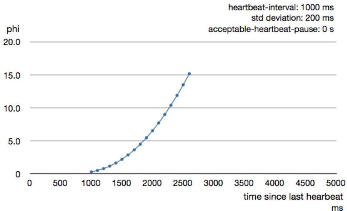
Phi is calculated from the mean and standard deviation of historical inter arrival times. The previous chart is an example for standard deviation of 200 ms. If the heartbeats arrive with less deviation the curve becomes steeper, i.e. it is possible to determine failure more quickly. The curve looks like this for a standard deviation of 100 ms.
