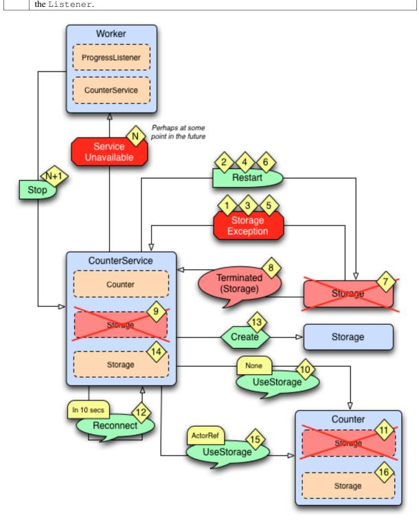
The above diagram illustrates what happens in case of storage failure. Failure flow:
