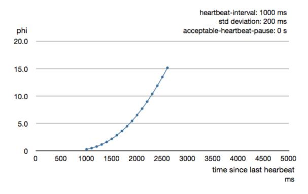
Phi is calculated from the mean and standard deviation of historical inter arrival times. The previous chart is an example for standard deviation of 200 ms. If the heartbeats arrive with less deviation the curve becomes steeper, i.e. it is possible to determine failure more quickly. The curve looks like this for a standard deviation of 100 ms.
